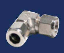
Compression Elbow NI Plated Brass 9.53 mm internal diameter 9.53 X 9.53 mm Tested up to 180 bar
